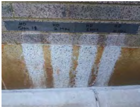
Granite cleaning tests
